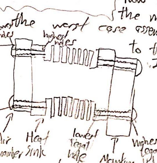
First, I'll evaluate the 2 4-40 screws connecting the mounting block to the heat sink. I've already accounted for the clearance holes being as high as possible on the mounting block, so now I'll account for the size of the screws relative to the clearance holes. For my bone tolerance calculation on page 1, I assumed MMC of these holes ( $\min \phi.115$ ), so I'll stick with that since in a single scenario, one feature maintains the same dimensions → K continued on next page
